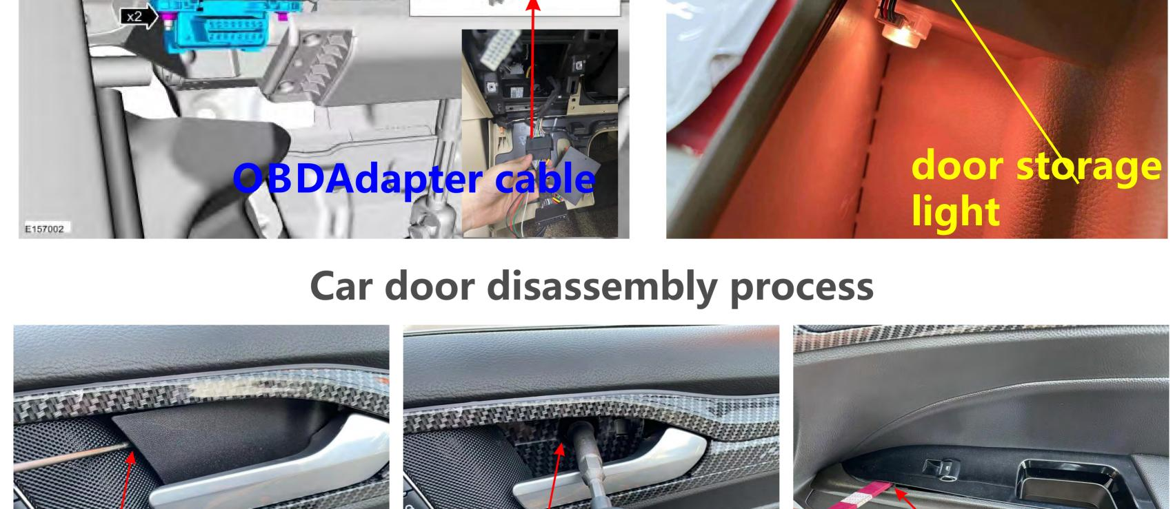
After taking off the cover, unscrew the screw
